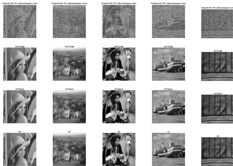
Fig. 6. Blurred images with 70% ratio (first row), rsetoration by FHITCGM-N (second row), rsetoration by HTHSLS (third row), rsetoration by HZ (bottom row).
