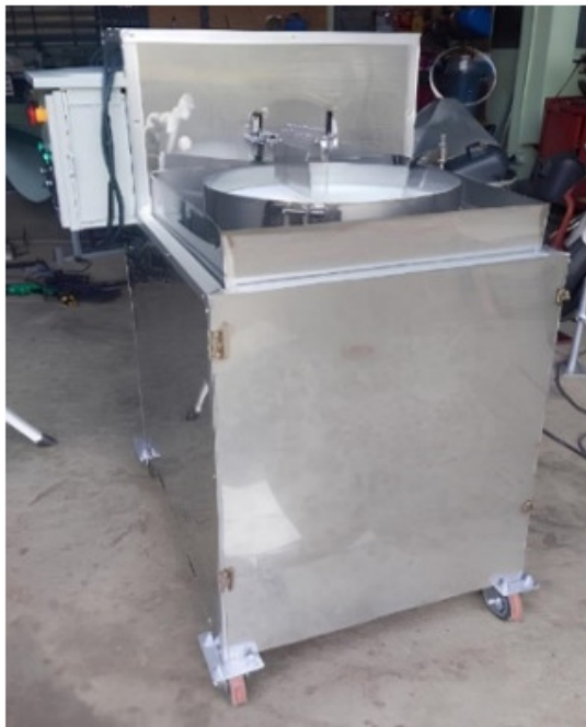
Fig. 3. A prototype of the fermented fish chopper machine.
