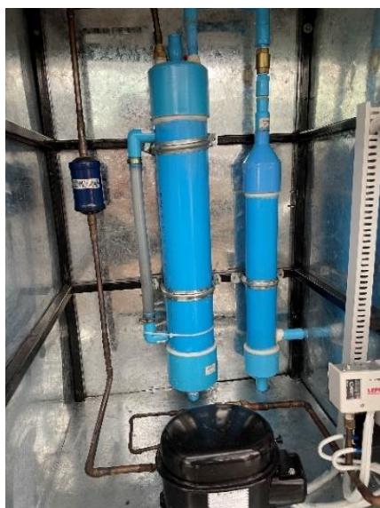
Fig. 8 Complete scrubbing and gas compressor for biogas in OTOP Duang Thong District
