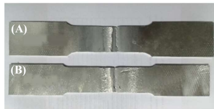
Figure 8 Fracture specimens of (A) MIG RW and (B) TIG RW of the AA 6082-T6.
